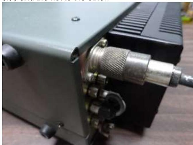
In a pinch, to operate your 80meter dipole on 160, back off the nut and feed the antenna with just the center pin. One step better is to connect the center pin and nut on the coax together and then connect the center pin to the rig. *Your mileage may vary as will the amount of RF in the shack.*
