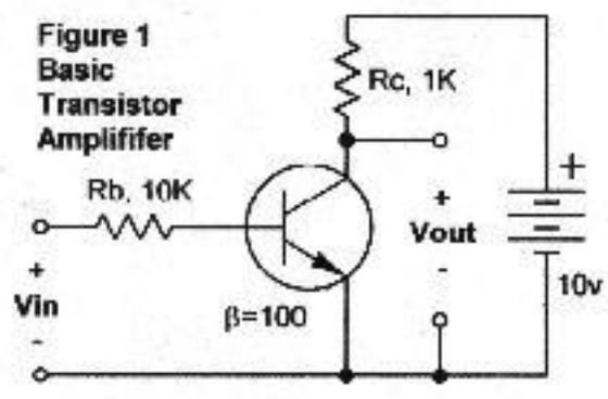
**Figure 1** shows the essentials of a transistor amplifier. When  $V_{in}$  is less than 0.7 volts, no current flows in the base, and therefore no current flows in the collector. This is called *cutoff*. By Ohm's Law, zero current means the voltage drop across  $R_c$  is zero, so 10 volts appears across the transistor as  $V_{out}$ .
