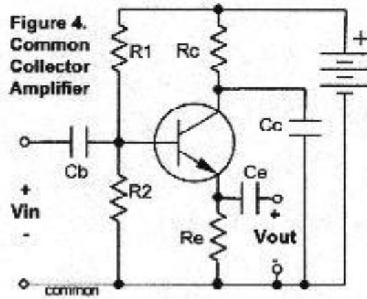
**Figure 4** shows a variation on this amplifier. Instead of bypassing the emitter to common, take the output signal from the emitter, and bypass the *collector* to common. This *common collector* amplifier is also called an *emitter follower*. Its advantage is that it has a very high input impedance, and very low output impedance. It is a *noninverting* amplifier: the output is *in phase* with the input.
