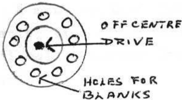
An eccentric drive is placed off centre, which when rotated allows the blanks to travel the entire width of the plate as shown above. Another cast iron plate is placed on top of the plate and the drive is started which begins to grind the quartz down.
